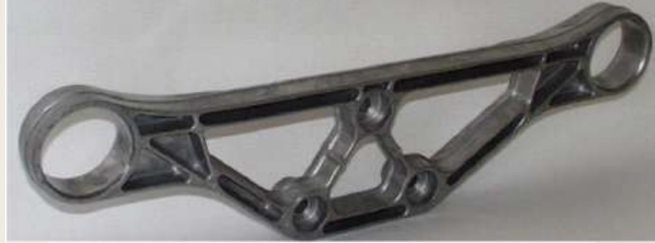
New design based on the topology optimization results
